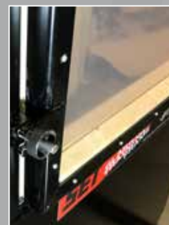
Different layers of glass or plastic sheets can be mounted to simulate various types of windows.
