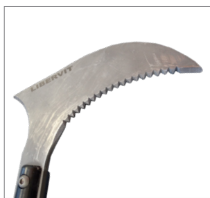
serrated cutting edge and spike
