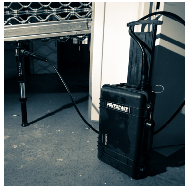
POWERCASE: hydraulic unit in a case
